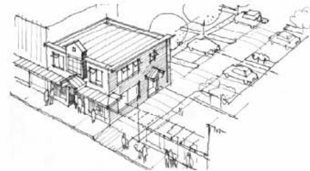
MAXIMISE MAINSTREET CONTINUITY - Providing parking behind uses accessed by narrow lanes (4m maximum width) can minimize disruption of street-based business uses. This helps maintain pedestrian amenity.
